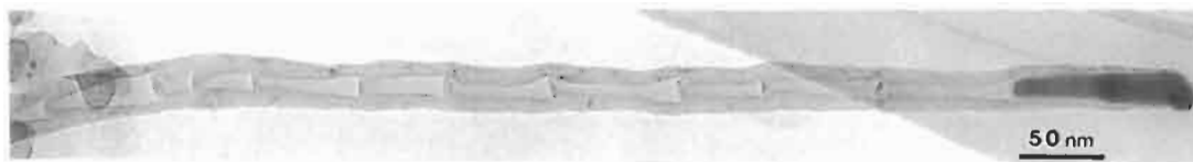
Fig. 8. TEM picture of a bamboo-shaped carbon tube.
