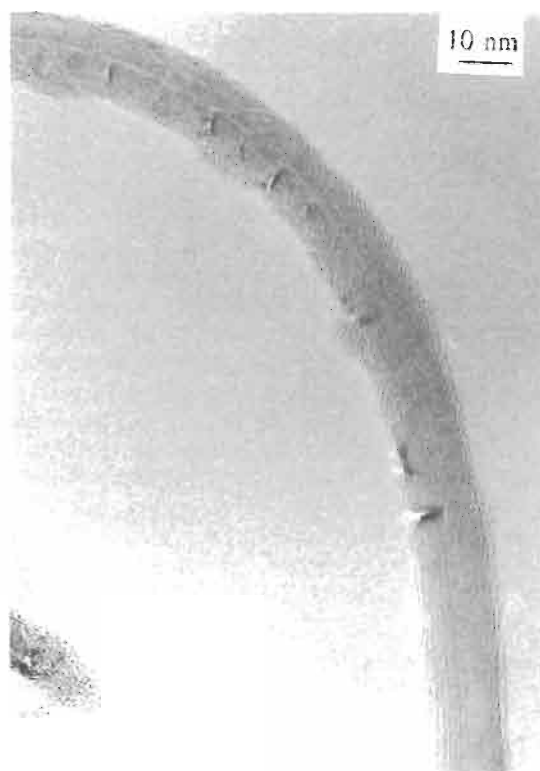
Figure 3. Lattice fringes LF 002 of buckled nanotube particles.
